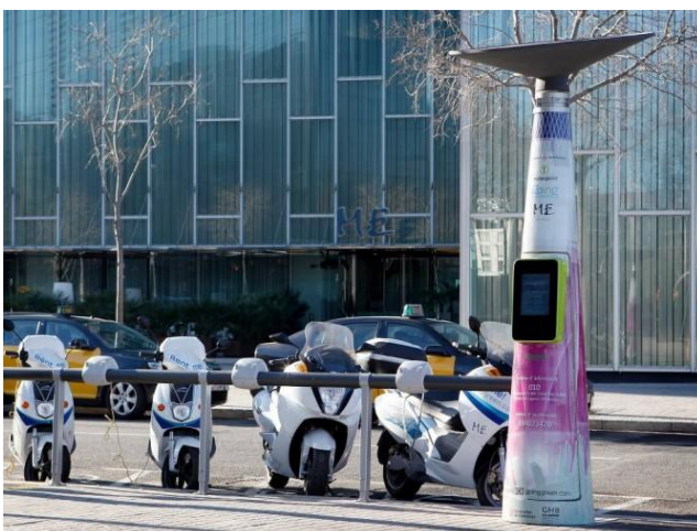
Mobecpoint, e-motorbikes charging station. Source: mobecpoint.com
